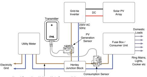
Normal Convention with Live cable to Consumer Unit being the right most cable connected to the Meter (Brown or Red normally covered with Grey sheath)
