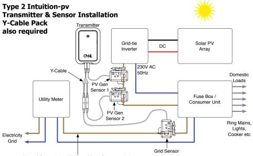
Normal Convention with Live cable to Consumer Unit being the right most cable connected to the Meter (Brown or Red normally covered with Grey sheath)
